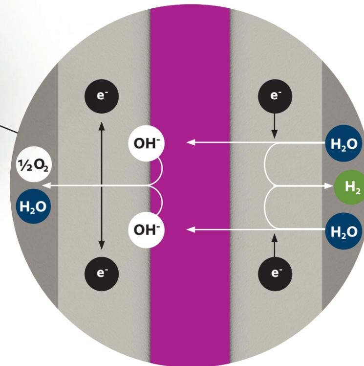
The DURAION® Membrane is the center piece in the electrolyzer with its ability to conduct anions. It separates the two reaction chambers and enables thereby the continuous production of hydrogen in the electrolysis cell. Multiple electrolysis cells are combined to a stack to increase the amount of hydrogen produced.
